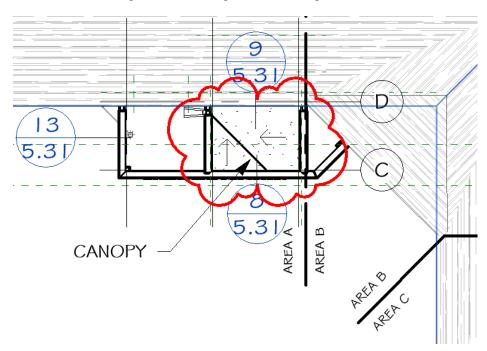
b) Provide tapered insulation at new Elementary/Middle School entry canopy in Area B per roof plan below. Starting thickness 1" at downspout location. Slope insulation ¼" per foot.
